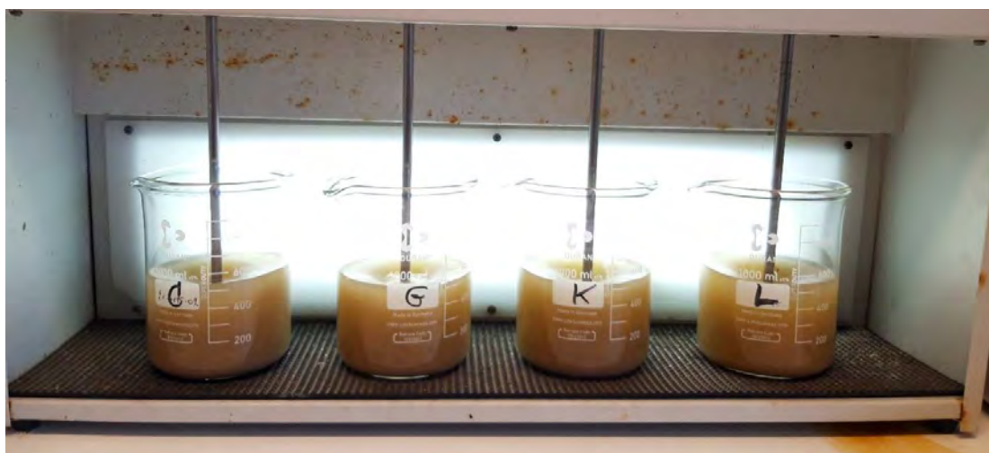
Figure 10. Sand samples during chemical washing
