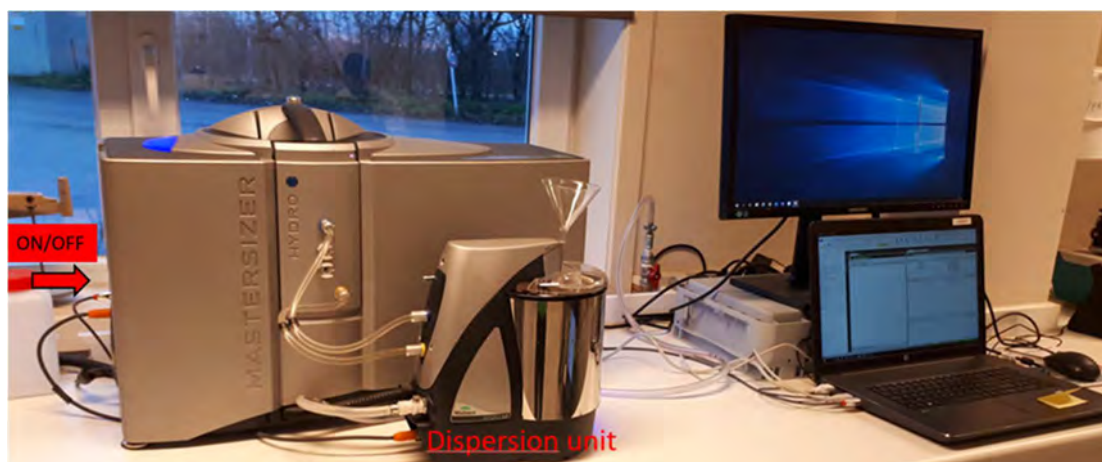
Figure 3. Laser diffraction apparatus Malvern Mastersizer 3000.
