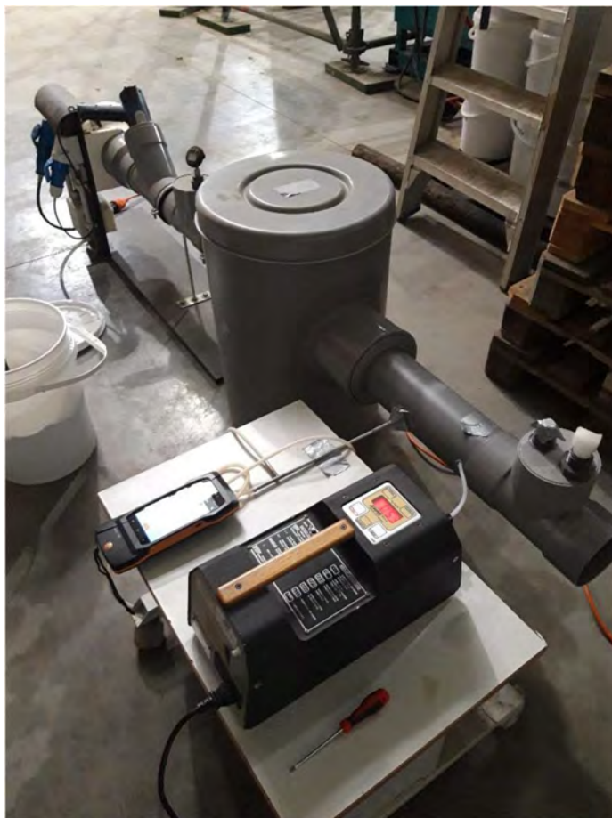
Figure 16. Emission flux chamber with mercury analyser.
