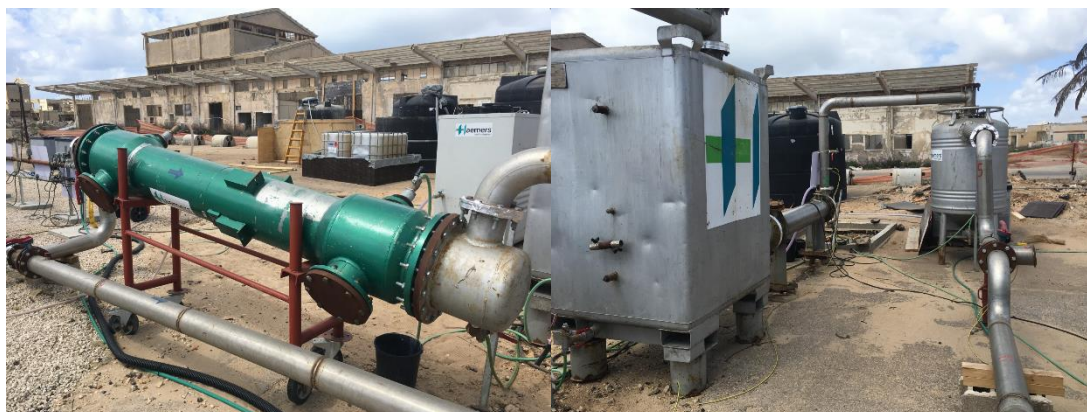
Figure 34. First heat exchanger of the VTU for the AKKO pilot process
