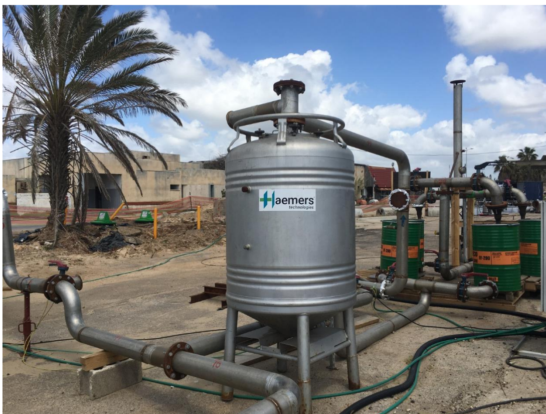
Figure 36. Knock-out to recover the condensate entrained in the flow
